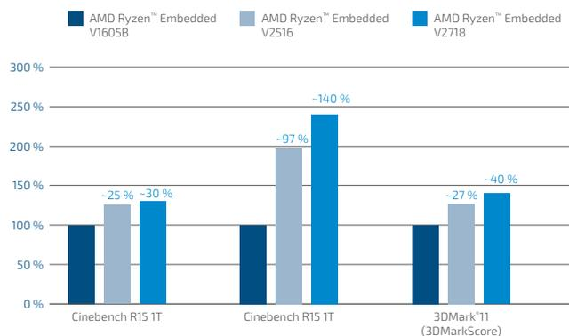
// The new AMD Ryzen™ Embedded V2000 processors offer another significant increase in performance per watt.
