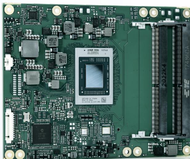
// The COM Express® Basic module offers a soldered NVMe SSD for up to 1 TByte of fully integrated, extremely robust and fast onboard storage.
