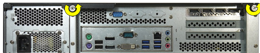
Figure 22: Loosen the knurled Screw on the Rear Side
