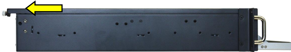
Figure 23: Pulling the Cover backwards
