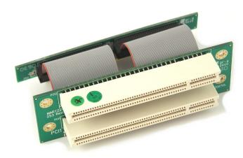
The spacing between the two PCI slots is 20.3 mm and the height above PCB of the PCI slots is 15.5mm. The position of the PCI-slots pin 1 (in mm) are: PCI1-[X, Y] = [17.2, 16.8] and PCI2-[X, Y] = [17.2, 37.1]. Between the two PCI slots there is a dual pin-row connector for selecting the AD number. The four mounting holes have Diameter 3.2mm.
