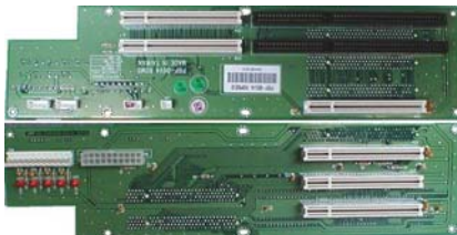
Fig. 20b: PICMG 1.0 Butterfly backplane for PCI-759SBC card
