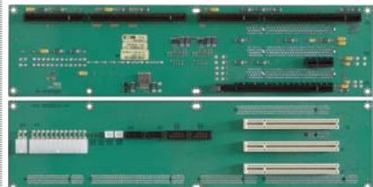
Fig. 20c: PICMG 1.3 Butterfly backplane for PCI-760/-960 SBC card
