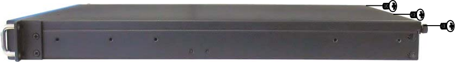
Fig. 30: Loosening the three knurled screws on the rear side of the KISS 1U system
