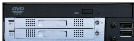
Fig. 15: Configuration example with a DVD Slim drive (L1) and a RAID1 slim drive for 2x 2.5" SATA HDD (L2)
