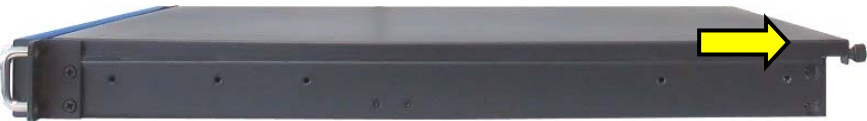
Fig. 31: Sliding the cover back will pull out the cover fixing brackets from the retaining brackets of the chassis.
