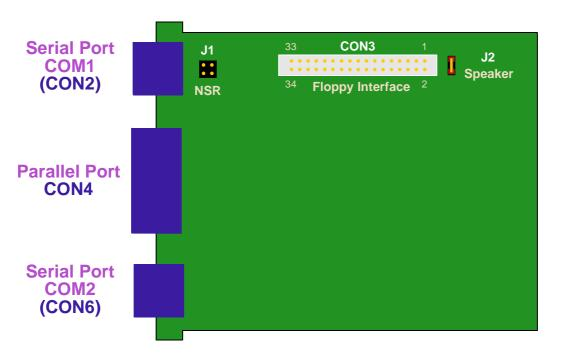
Figure C-1: IDE2 Module Layout, Standard Version (Front Side)
