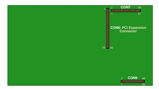
Figure B-3: PMC Module Layout, Version with CPCI Connectors (Front View)
