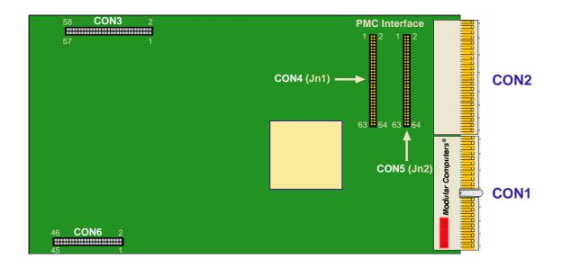
Figure B-4: PMC Module Layout, Version with CPCI Connectors (Rear View)
