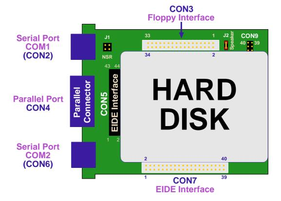
Figure C-4: IDE2 Module Layout, HardDisk Version (Reverse Side)
