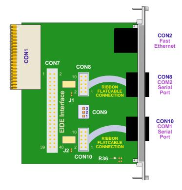
Figure D-3: CP-RIO3-01 Module Layout, 8HP Version
