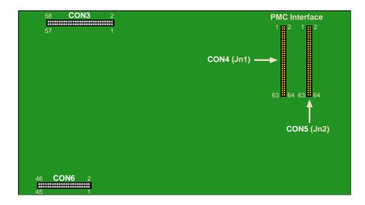
Figure B-2: PMC Module Layout, Version without CPCI Connectors (Rear View)
