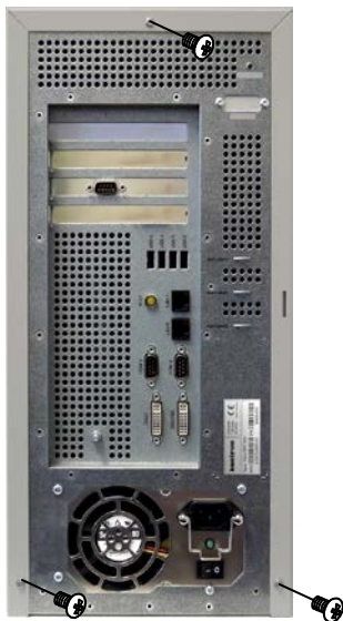
Fig. 9: Loosen the fastening screws on the rear side of the Clinic DPC 210 system
