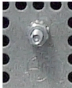
Fig. 7: Detail grounding stud marked with “PE” symbol
