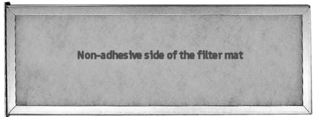
Fig. 21: How to insert the filter mat into the holder
