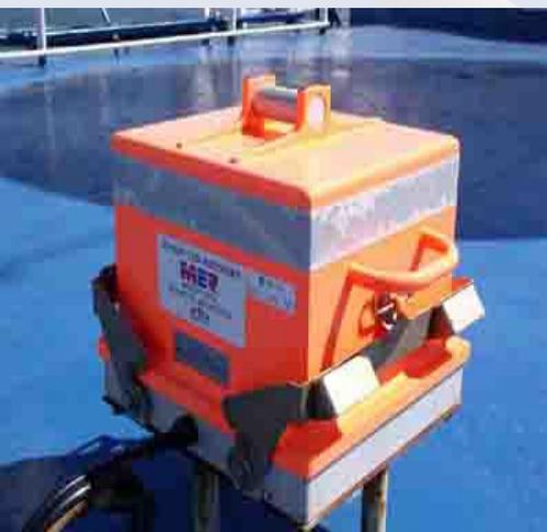
The inside of these deep sea-suited boxes is loaded with high-tech electronics, which can record several GB of data from heterogeneous sources and store them for more than 12 hours. For example, a special rule algorithm stops the recording at the time of a collision so that the crucial event window remains documented. Thus, the stored data offers the basis for a realistic and objective evaluation.
