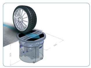
Image 2: Via laser diode-digital cameras, which are fit into shafts in the highway or troughs, tire treads depths can be captured and calculated in milliseconds by the integrated DIN rail PC, Kontron ThinkIO.
