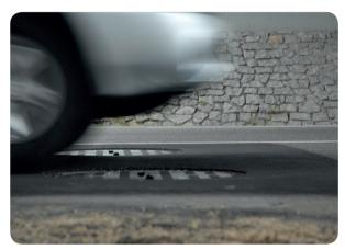
Image 1: The image processing system ProContour H3-D measures tire tread depths at up to 120 km/h in moving traffic
